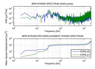
Figure 3: The power density of 4kHz BPM data corresponding to  $D_x=0.5~{\rm m}$  with FOFB on or off. Data taken with 100 mA beam.
