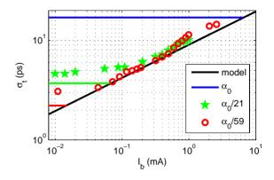
Figure 5: Measured bunch length in the two low alpha modes and the model calculation according to Ref. [8].
