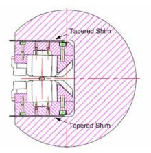
Figure 5: Tapered shims are moved horizontally to adjust the undulator gap.
