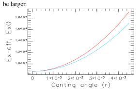
Figure 3: The natural and effective horizontal emittance as functions of the canting angle.
