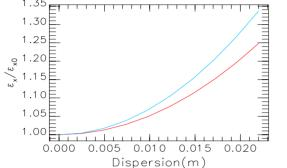
Figure 1: The horizontal emittance growth ratio as a function of external dispersion in the straights. The blue line is for the effective emittance, and the red line is for the horizontal emittance  $\epsilon_{x,0}$ .
