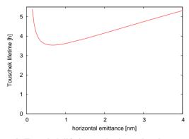
Figure 3: Touschek lifetime vs horizontal emittance.
