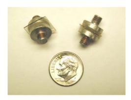
Figure 5: SiC photoconductive switches. Each wafer is approximately 400  $\mu$ m thick A-plane material with copper electrodes bonded on opposite sides.
