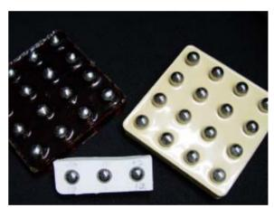
Figure 6: Samples of the cast dielectric material. The brown color material has a low relative dielectric constant  $(\approx 3)$  while the light colored material has a high concentration of nanoparticles with a relative dielectric constant of approximately 40.
