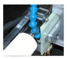
Figure 4: Blumlein with self-breaking oil switch. The line uses sheet insulation of biaxially oriented polypropylene (BOPP) with a total thickness of 2.5 mm per line. The assembly is immersed in degassed oil and can be charged to over 250 kV without breakdown.
