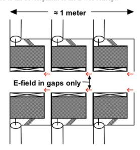
Figure 1: Conventional induction accelerator structure showing three induction modules. The walls are metallic and accelerating fields appear only across the relatively small vacuum gaps. Most of the cell volume is taken up by a magnetic core.
