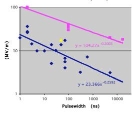
Figure 3: Plot showing surface flashover field stress as a function of pulsewidth for conventional (monolithic) straight wall insulators culled from the literature along with HGI data points showing increased performance.
