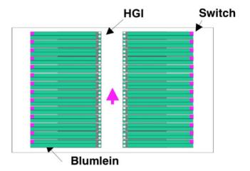
Figure 8: Blumlein stacks surround an HGI. The entire assembly can be enclosed in a metal case without shorting out the voltage if the spatial extent of the excitation on the wall is less than the axial length of the case. Under those conditions the unfired lines act as series loads to the switch end of the Blumlein stack and prevent the collapse of the voltage at that end of the line.
