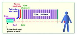
Figure 9: A spark discharge source provides the protons through a small aperture. Extraction and focusing electrodes are used to control intensity and spot size.
