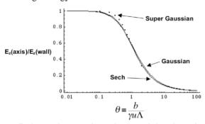
Figure 7: Approximate universal curve giving the ratio of on-axis electric field to that along the beam tube wall as a function of the dimensionless parameter  $\theta$  for several different temporal wave shapes.
