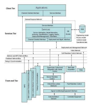
Figure 1: Controls systems functional model.
