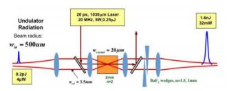
Figure 4: Layout of the optical amplifier.
