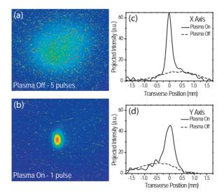
Figure 2: Images of the unfocused (a) and focused (b) electron beam OTR displayed with the same scaled to intensity color map. In order to provide sufficient contrast, the unfocused image (a) is the integration of 5 beam pulses. The projected intensity of the focused and unfocused beams (normalized to 1 pulse) in the x axis (c) and y axis (d) is also shown.
