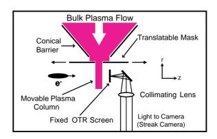
Figure 1: Schematic of the plasma lens apparatus.
