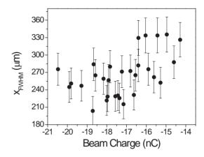
Figure 4: Dependance of the focused beam spot size on the beam charge under otherwise similar conditions.
