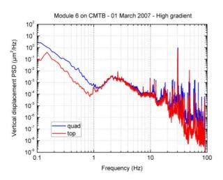
Figure 6: PSDs measured on vessel top and on quad during high power RF tests: the klystron was running at 10 Hz and the average gradient achieved was ~27 MV/m.
