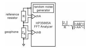
Figure 1: Block diagram of the calibration setup.
