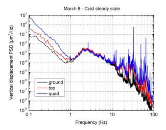
Figure 5: PSDs of ground, vessel top and quadrupole in cold steady state with RF off, measured just after reaching the cold stable conditions at the end of the 11<sup>th</sup> cooldown.
