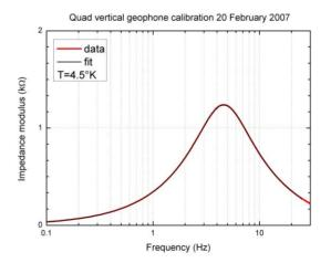
Figure 2: Calibration curve of the vertical geophone measured at 4.5 K during the test run of Module 6.
