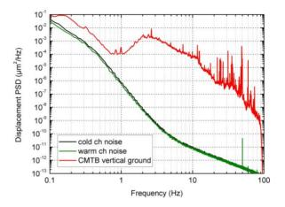
Figure 3: Comparison between the noise of the data acquisition system (amplifier+ADC) and the vertical ground spectrum measured at CMTB in the morning of a working day.
