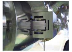
Figure 6: Cavity sliding fixtures
