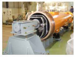
Figure 7: Insertion into the vacuum vessels
