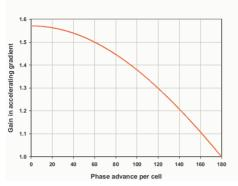
Figure 2. The gain in the accelerating gradient of the traveling wave accelerating structure compared to a standing wave  $\pi$ -structure versus the phase advance per cell for the ideal case. For  $\pi/2$  the gain is  $\sqrt{2}$ , or 42%.
