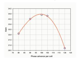
Figure 3. The gain in accelerating gradient versus phase advance per cell. The aperture is 60 mm, and the diaphragm thickness is chosen to be not less than 11.5 mm.
