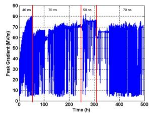
Figure 2: Conditioning history of HDX11 molybdenum structure.
