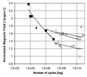
Figure 2: Fatigue curve for OFE-copper (full diamond, laser; empty diamonds, ultrasound), CuZr (full squares, laser; empty diamonds, ultrasound) and Glidcop (crosses, ultrasound). Arrows indicate samples which did not fracture. Materials are in the state as in table 1. The vertical axis is the equivalent amplitude of the RF magnetic field corresponding to the applied stress amplitude. It is normalized to 1 corresponding to the target value (triangle) for a CLIC design with  $\Delta T$ =56K.
