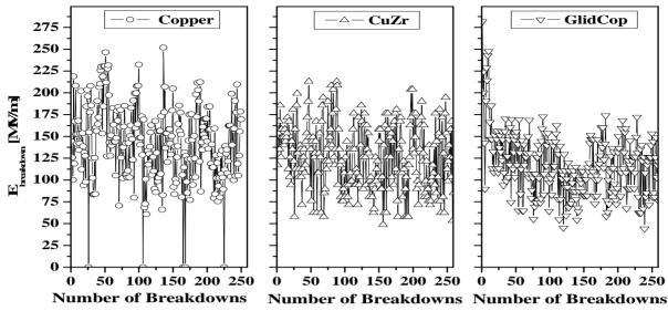
Figure 1: Comparison of the conditioning in DC breakdown experiment for OFE-Copper, CuZr, and Glidcop AL15.
