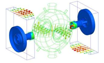
Figure 1: Simulation results of the cavity/two-coupler model showing vector plots of the cavity magnetic fields and properly phased electric fields in the input waveguide feeding each coupler. The contour plot shows the relative power density along the body of the coupler.
