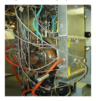
Figure 5: Photo of test cavity fitted with two input couplers.
