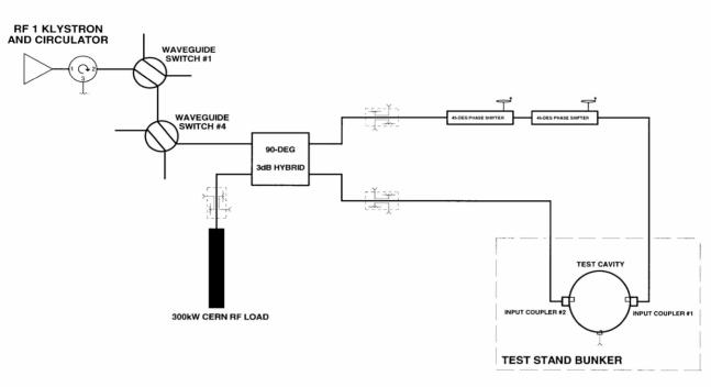
Figure 2: The two-coupler test system.
