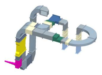
Figure 3: Drawing of the dual-feed waveguide system.
