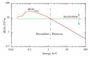
Figure 1: Drag and acceleration terms as a function of particle energy for a 1 g/cm<sup>3</sup> material.
