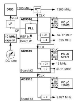
Figure 3: Master oscillator block diagram.
