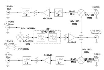
Figure 2: Block diagram of the 13 MHz IF receiver [7].
