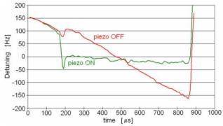
Figure 1: Cavity resonance frequency shift induced by Lorentz forces, without (red) and with (green) piezo compensation.
