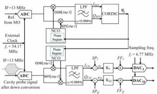
Figure 4: Digital down conversion scheme, performed by the SIMCON FPGA [6].
