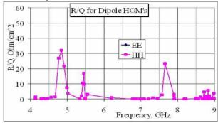
Figure 2: Calculated R/Q of the 9 cell 3<sup>rd</sup> harmonic Cavity.
