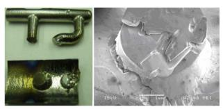
Figure 3: Curved leg of the HOM F-probe fractured from HOM can.
