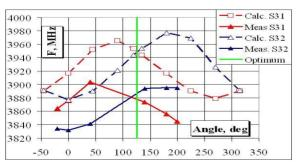
Figure 8: Notch frequency vs. position of the HOM coupler version-4.
