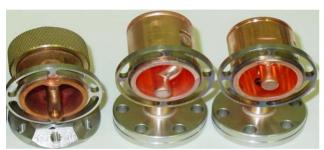
Figure 7: Copper mockups of the HOM couplers. Left is old design, in the middle version -2, right version -4.
