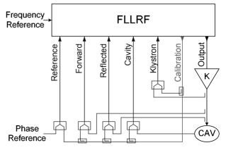
Figure 2: Fermi LLRF control system configuration.
