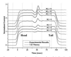
Figure 4: Comparison of experimental and 1-D simulation data for a -300eV pulse perturbation.
