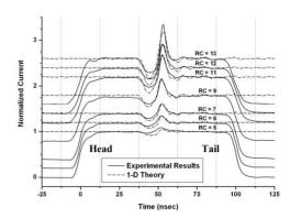
Figure 5: Comparison of experimental and 1-D simulation data for a -600eV pulse perturbation.
