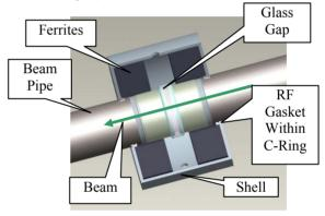
Figure 1: Pro-E drawing of the IM.
