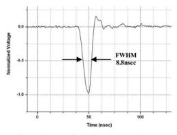
Figure 3: Negative pulse output voltage.
