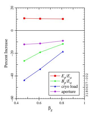
Figure 4. Figures of merit for half-reentrant cavities relative to elliptical cavities (SNS/RIA) as a function of geometrical  $\beta$ .
