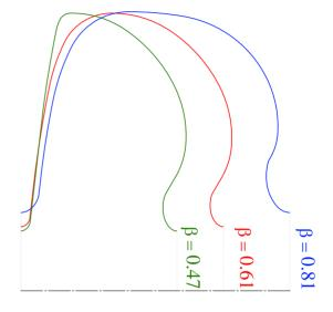
Figure 1. Cell shapes for reduced- $\beta$  half-reentrant cavities.
