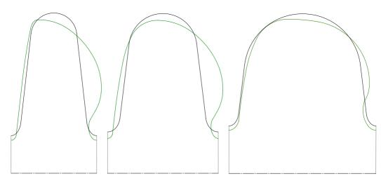
Figure 2. Comparison of cell shapes for non-reentrant cavities (RIA/SNS) and half-reentrant cavities. Left to right:  $\beta = 0.47$ ,  $\beta = 0.61$ , and  $\beta = 0.81$ .
