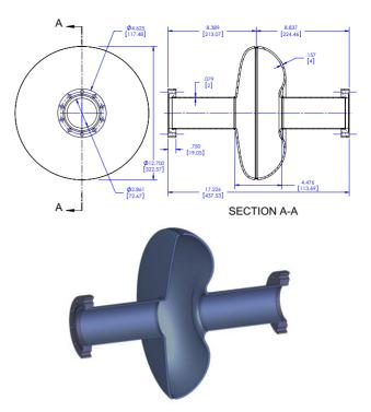
Figure 5. Two-view drawing (top) and isometric sectional view (bottom) of the 805 MHz  $\beta = 0.61$  single cell prototype.
