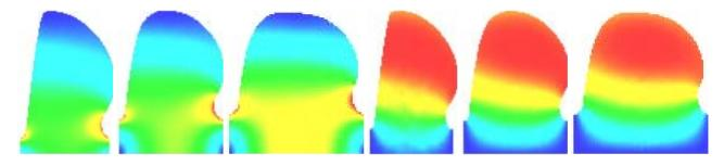
Figure 3. Electric (left) and magnetic (right) field maps for the half-reentrant cavities. Red indicates a large field magnitude and blue indicates a low field magnitude.
