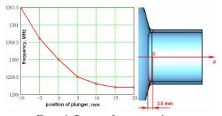
Figure 6: Resonant frequency tuning.
