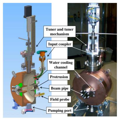
Figure 4: Cornell ERL injector deflecting cavity
