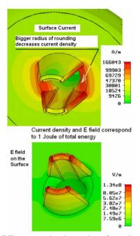
Figure 3: RF current density and surface electric field near the protrusions.
