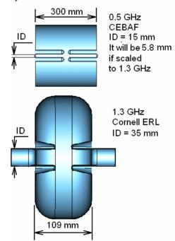
Figure 1: Comparison of the CEBAF and Cornell ERL deflecting cavity shapes.
