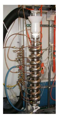
Figure 3: Vertical EP apparatus in operation
