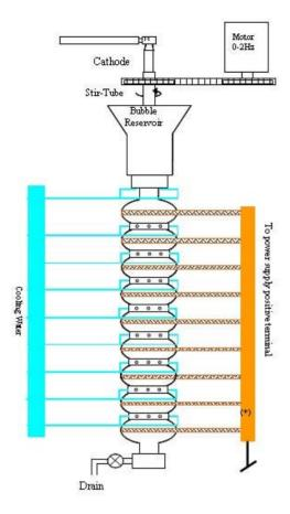
Figure 2: Laout of the vertical EP system
