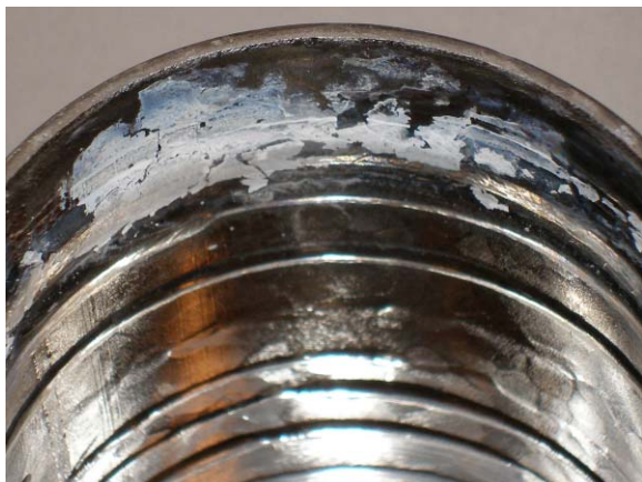
Figure 3: White and yellow deposit accumulated on the can after heavy electropolish.
