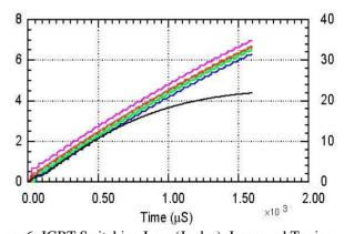
Figure 6: IGBT Switching Loss (Joules), Improved Tuning.
