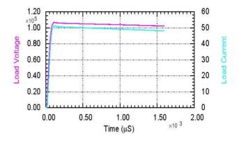
Figure 1: Unregulated Converter-Modulator Droop.
