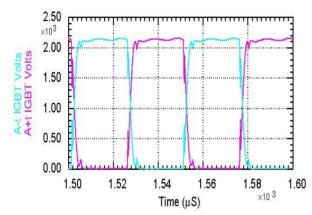
Figure 7: Improved Tuning Collector-Emitter Voltage.
