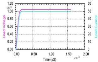
Figure 5: Flat-Topped Output (~.25%) with PWM.
