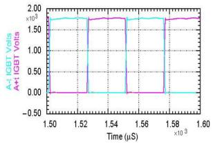
Figure 4: Totem-Pole Pair IGBT Collector-Emitter Voltages.
