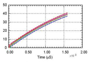
Figure 2: IGBT Switching Losses (Joules).
