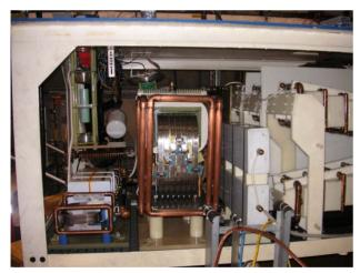
Figure 2: View of doubler capacitors and output filter choke
