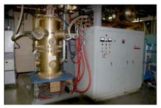
Figure 1: 201 MHz cavity amplifier and filament supply for the Burle 7835 triode.
