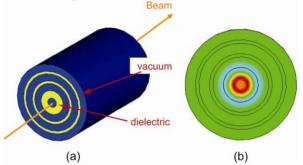
Figure 1: The schematic of an omniguide, the blue area is vacuum and the yellow area is dielectric (a); the longitudinal electric field magnitude in the TM01-like mode of an omniguide computed with Microwave Studio [6] (b).
