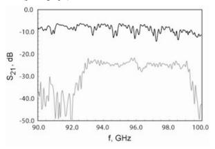
Figure 5: Measured transmission through the omniguide structure (black line). For comparison measured transmission through the LANL W-band vane-loaded TWT structure [3] is shown (grey line).
