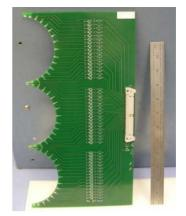
Figure 8: Fabricated 3-cell section board.
