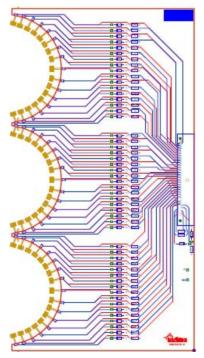
Figure 7: 3-cell section board layout.
