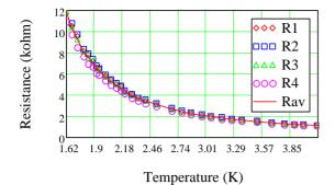
Figure 2: Temperature dependence of 4 Allen-Bradley resistors and its average value.
