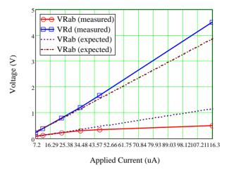
Figure 4: Measured and expected voltage from the self heating test (upper left circuit in Figure 3).
