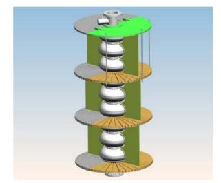
Figure 1: Solid model of a 9-cell cavity with 6 sensor boards attached.
