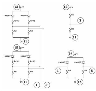
Figure 3: Prototype board. Left: power switching concept; upper right: self heating test; lower right: diodes operation test. RsA2 and RsB1 are Allen-Bradley resistors.
