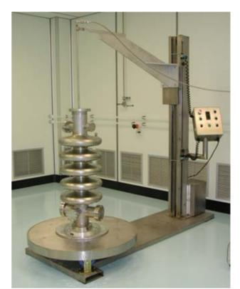
Figure 1: Automatic cavity rinsing station.
