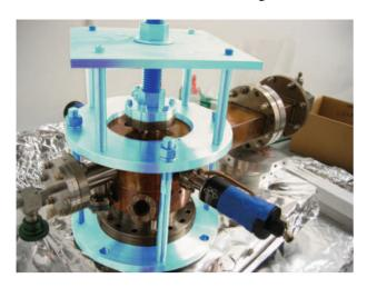
Figure 2: Stretcher device installed on photoinjector. Stretcher is artificially highlighted in photograph for clarity.
