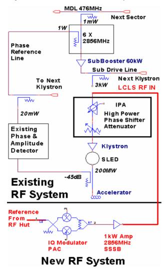
Figure 4: SLAC linac RF system and LCLS input.
