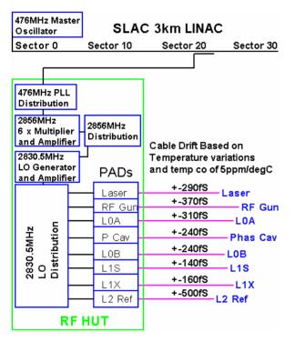
Figure 2: Reference and signal cables.
