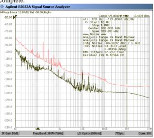
Figure 3: Phase noise spectrum of the LCLS oscillator, bottom, compared to Linac RF, Top 10 Hz to 10 MHz.
