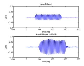
Figure 7: 100 ns RF tone burst Amplifier "B".
