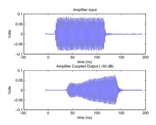
Figure 6: 100 ns RF tone Burst Amplifier "A".
