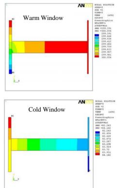
Figure 8: Temperatures in the warm and cold window, Warm and Cold Window Design, with RF
