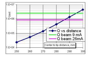
Figure 5: Qext: Triple Spoke Cavity. β=0.62, 79mm port.
