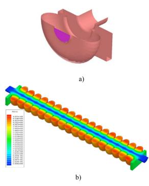
Figure 3: a) Transverse cuts through the rectangular waveguide coupling section for the L-band SCTW accelerating structure, side view; b) Magnetic field of the 18-cell SCTW cavity with the optimized coupling section.
