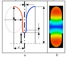
Figure 2: Cell geometry of the superconducting TW accelerating (STWA) structure: (a) STWA structure cavity shape; (b) magnetic field distribution in the STWA cell.
