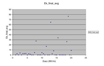
Figure 8. Multipacting analysis of the tapered outer choke section. The taper goes from 13 mm to 20 mm radius.
