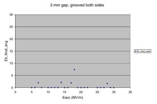
Figure 7. The results of the multipacting simulation on the choke joint design with grooves on all faces.
