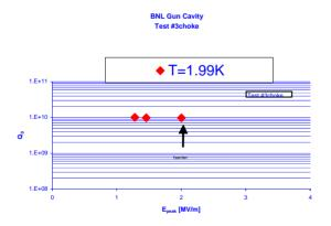
Figure 4. The performance of the original cavity with the cathode inserted.
