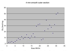
Figure 9. The multipacting analysis of a 4 mm wide outer choke joint that is smooth on both faces.
