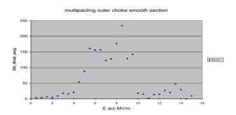
Figure 6. The multipacting analysis from the initial choke design.
