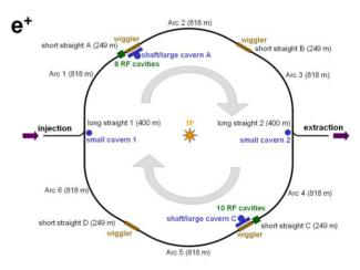
Figure 1: Layout of the positron damping ring.
