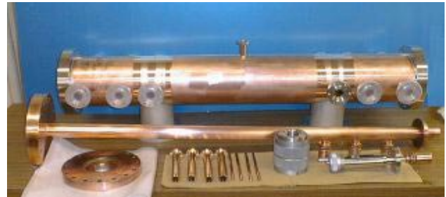
Figure 6: Proof of principle model for coaxial cavity.
