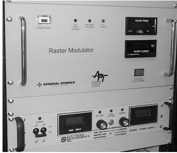
Figure 4: Photo of one modulator and ac/dc converter
