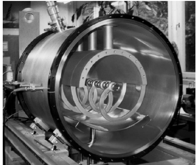
Figure 5: The 5.4% power type resonator prepared for low power rf measurements
