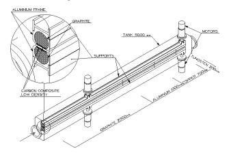
Figure 4: Perspective sketch of the TDI assembly (preliminary).
