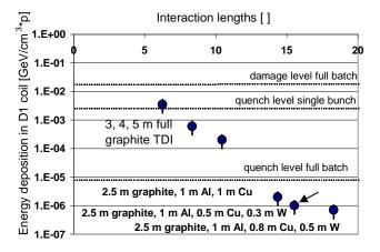
Figure 3: Energy deposition in D1 coil as a function of the number of interaction lengths of the TDI (case 1).
