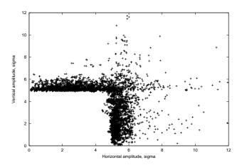
Figure 4: Proton beam halo in the Tevatron aperture.
