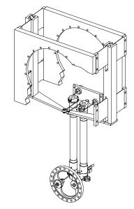
Figure 3: Tuner mechanism
