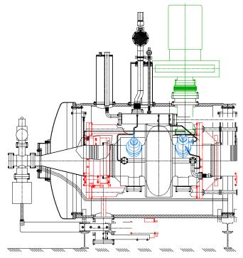
Figure 2: Partial view of the prototype cryomodule with two cavities (a series cryomodule has four cavities)
