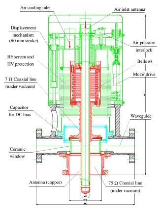
Figure 4: The LHC variable coupler
