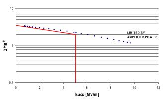
Figure 1: Typical cavity performance and acceptance curve
