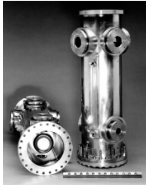
Figure 4: First two resonators complete with the stainless steel outer housings.
