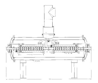
Figure 3: Cryostat module with two cavities.
