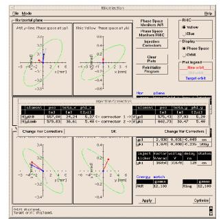
Figure 2: Graphical user interface for the injection tuning program showing the horizontal and vertical orbit and the lattice in the injection region. Active correctors and their settings are displayed.
