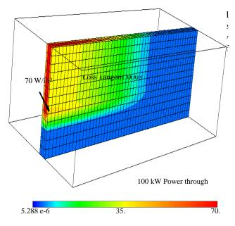
Figure 3: Heat loss contours determined by MAFIA
