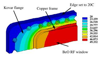
Figure 4: Temperature contours from ANSYS
