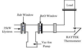
Figure 7: RF window test set up
