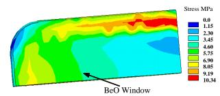
Figure 6: Von Mises stress of the BeO window
