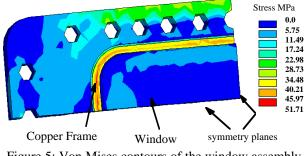
Figure 5: Von Mises contours of the window assembly
