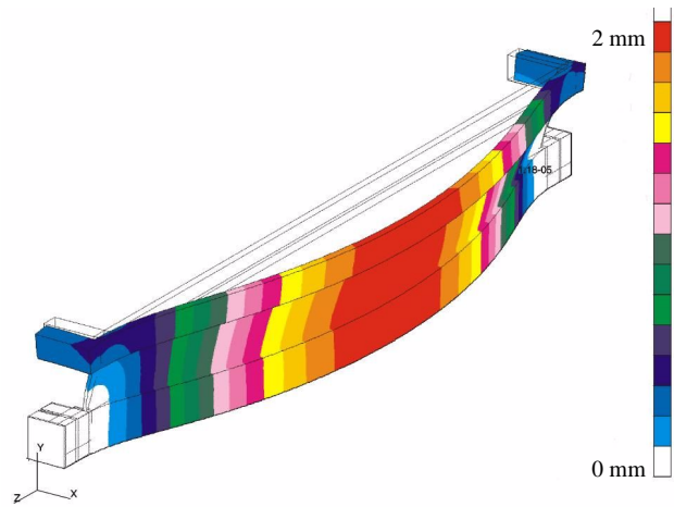
Figure 5: Deformation of the mechanical support structure due to thermal expansion.
