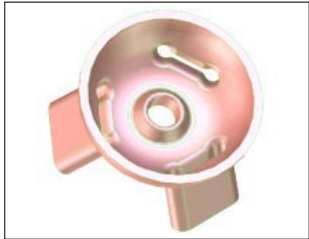
Figure 3: 3-D engineering sketch of half-cavity showing ridged damping waveguides, beampipe, and nose cones.
