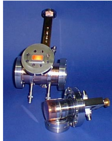
Figure 1: Picture of test cavity with one of the endcaps in the foreground.
