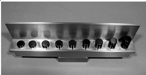
Figure 4: Cut-away view of the SiC-dummy-load. The SiC-ceramic absorbers brazed on the narrow wall (3.4-cm) of the conventional S-band rectangular wave-guide are black in color. All the SiC-ceramic absorbers have the same 2-cm diameter.
